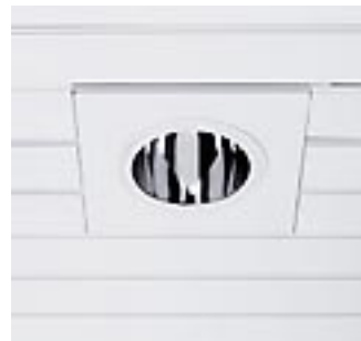
82954.000 Mounting plate for panelled ceilings Metal, white (RAL9002) powder- coated. Module 100 (85/15, 84/16). For downlights with ceiling aper- ture Ø 214mm. Recessing dimension 287x287mm.
